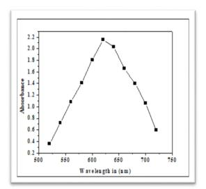
Fig. 2: Absorption spectrum of Azathioprine with MBTH /FeCl<sub>3</sub>
