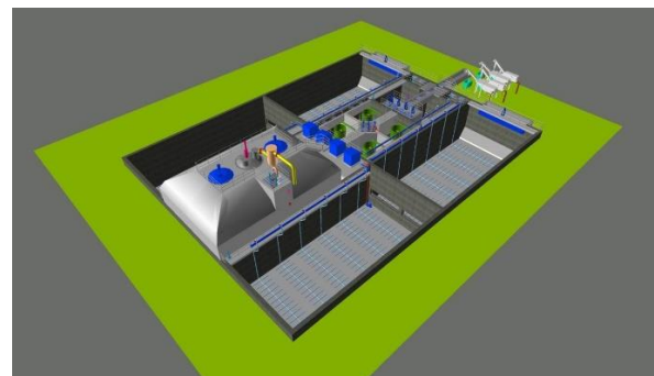
Figure 5. DUPLEX-technology for energetic autarkic treatment of wastewater and solid waste
