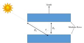
Figure 4. Top view of tilted PV row
