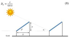
Figure 3. Side view of tilted PV row
