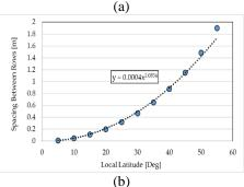
**Figure 5.** Average spacing between two rows for 5° to 55° local latitudes: (Left) winter solstice (Right) equinoxes
