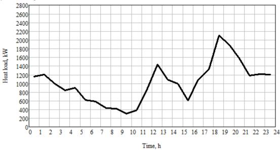
Figure 7 – Total heat load on the refrigeration system with cooling towers
