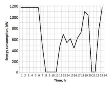
*Figure 5* – *Energy consumption diagram for refrigeration system with accumulation*
