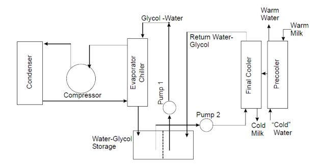
Figure 1 – Instant milk cooling system with decoupled, two pump, system
