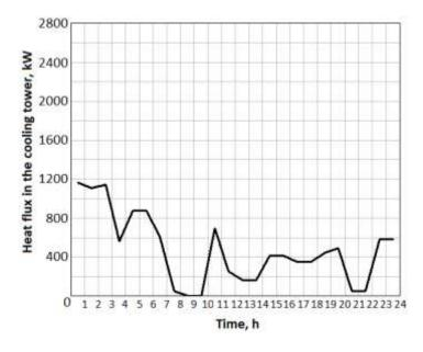
Figure 6 – Amount of heat that could be withdrawn with cooling tower
