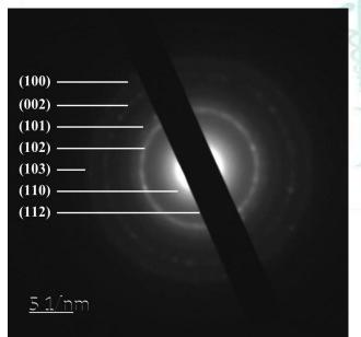
Figure 3: TEM of ZnO nanogel consisting Nanoparticles
