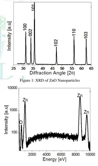
Figure 2: EDS spectra of ZnO nanoparticles
