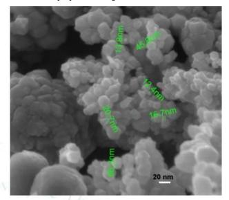
Figure 4: SEM of ZnO Nanoparticles
