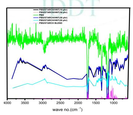
Figure 1: FTIR Analysis of PBS/Starch/Halloysite composites
