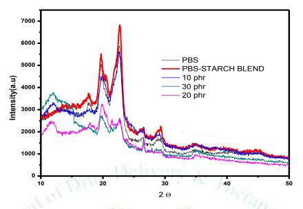
Figure 2: XRD Study of PBS, PBS/Starch blend and PBS/Starch/HNT composites.
