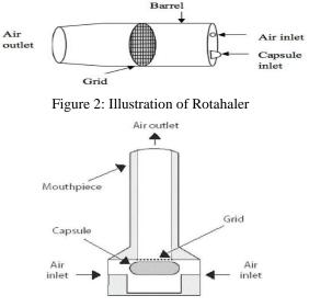
Figure 3: Illustration of Aerolizer
