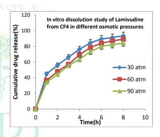
Figure 10: *In vitro* release profiles showing Lamivudine release from best CF4 in different osmotic pressures
