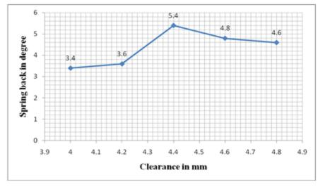
Figure 8: Graph of clearance and spring back
