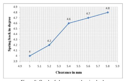
Figure 9: Graph of clearance and spring back
