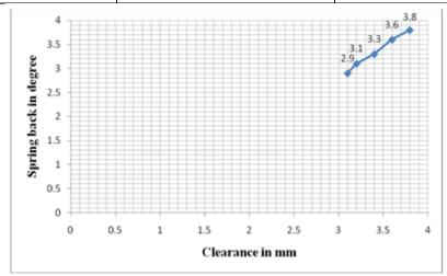
Figure 7: Graph of clearance and spring back
