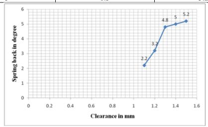
Figure.5. Graph of clearance and spring back
