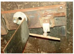
Figure 3: sheet metal clamping mechanism
