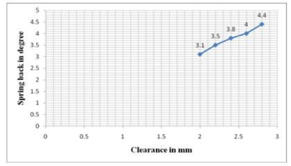
Figure 6: Graph of clearance and spring back
