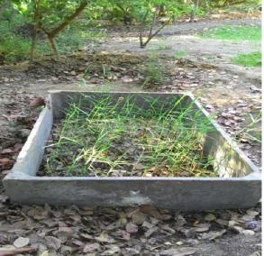
Wetland Vegetation: The study was carried out with Phragmites karka plants, which are grown in round shaped gravel filled in constructed wetlands. It was collected from local natural wetland and transplanted on the same day in a bucket filled with water and maintained for a period of 5 days to remove all previous impurities from the roots. These plants were transplanted from bucket to constructed wetland unit open to atmosphere in the park. The 5-6 cm spacing was set between the plants.
