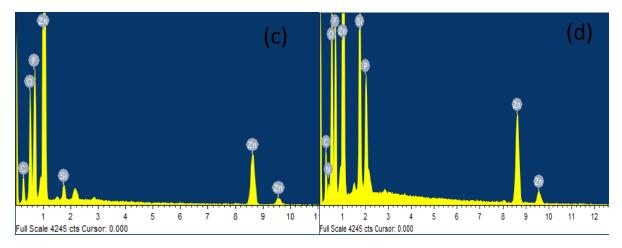
Fig. 3 EDX pattern of as prepared CdS nanoparticles and ZnO nanoparticles in various ILs (a) CdS in [EMIM] BF4 (b) CdS in [EMIM] PF6 (c) ZnO in [EMIM] BF4 (d) ZnO in [EMIM] PF6
