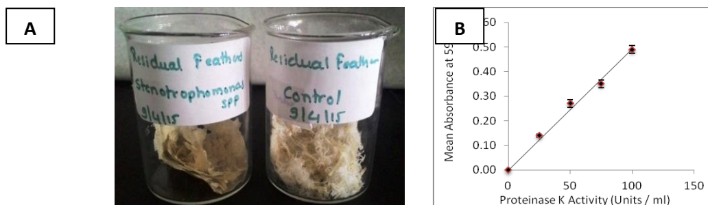
Figure 1: A Residual feathers after treatment with Stenotrophomonas maltophilia K279a; B – Standard Proteinase K graph using Keratin Azure k 8500 as a substrate.
