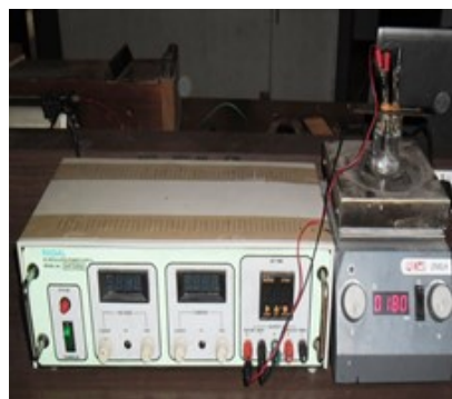
Fig 1. Electro-deposition Setup in the laboratory
