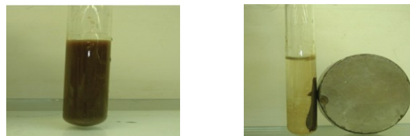
Fig. 7 Separation of catalyst using an external magnet.
