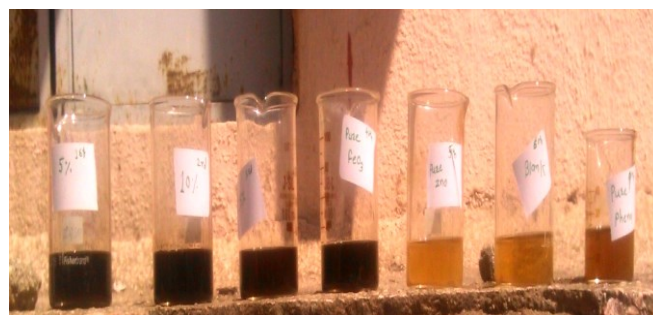
Figure 9: Photographs of phenol degradation process a)5% b) 10% C) 15% d) pure FeO e) pure ZnO f) blank g) Pure phenol after 120 minutes
