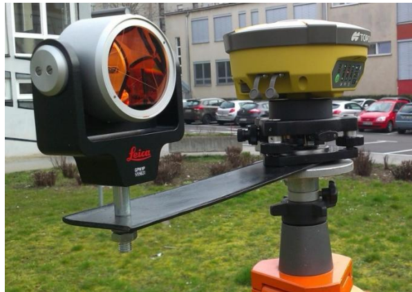
Figure 6: Hiper V and GPH1P prism on a tripod
