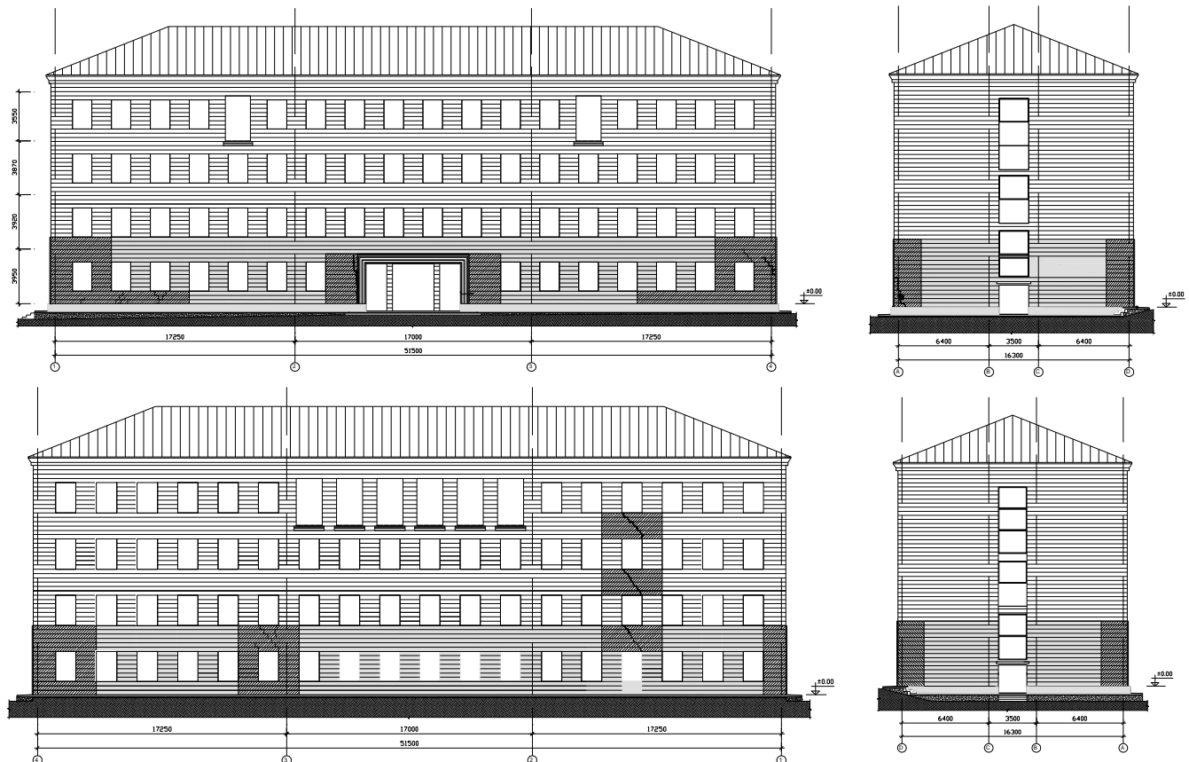
Figure 2: Main, side, and back façades of the 4-story old damaged stone building of the school #68 indicating damages and the designed R/C jackets
