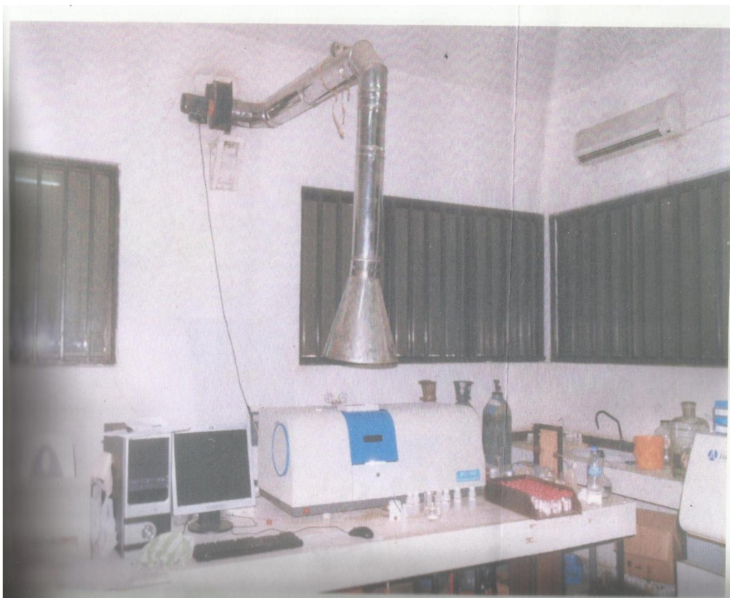
Figure 1: Atomic absorption spectrophotometer and 57 samples
