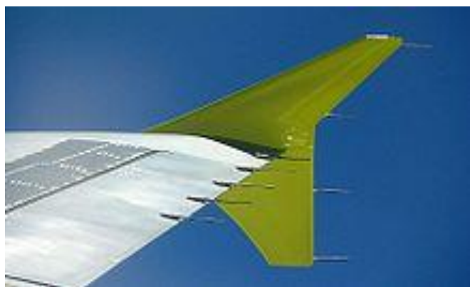
Figure. The AT winglet wingtip of the Airbus A319
