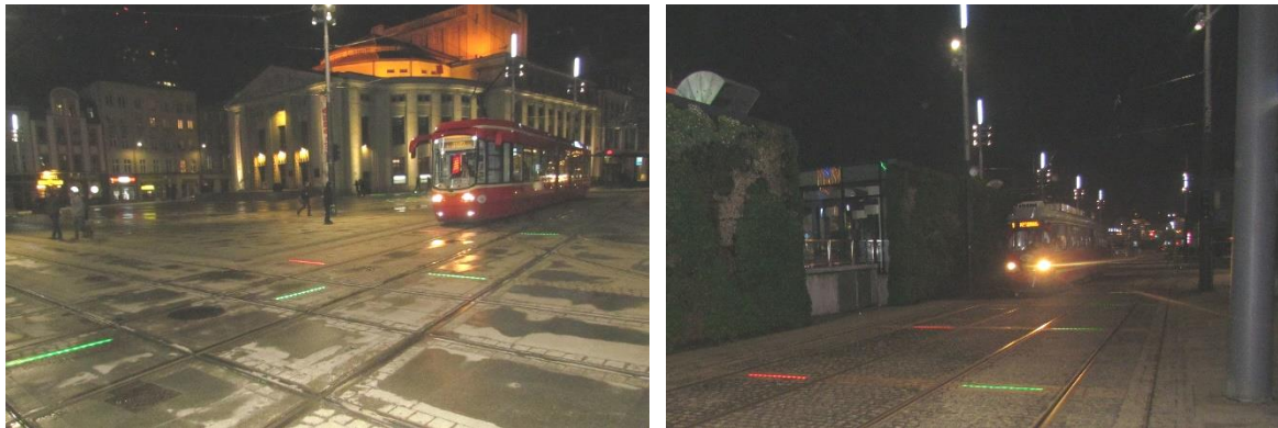
Fig. 6. Lights warning pedestrians of an incoming tram (source: own research)
