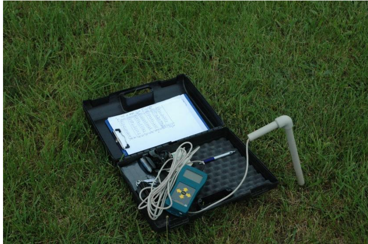
Fig. 3. A handheld TDR moisture meter used for grass runway monitoring
