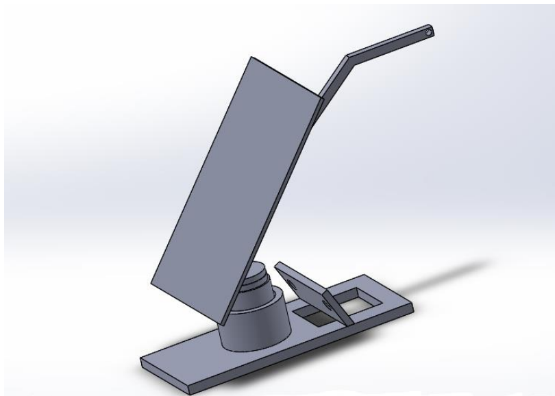
Fig. 1. The work of an accelerator pedal with an applied device mounted on the original flat bar of the cabin floor
