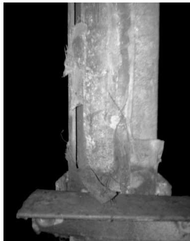
Fig. 1. Portions of the corroded filter on the measuring tube of the storage fuel tank
