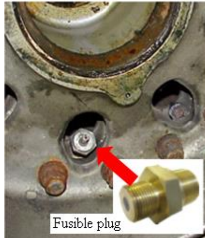
Fig. 2. Fusible plug on the wheel disc
