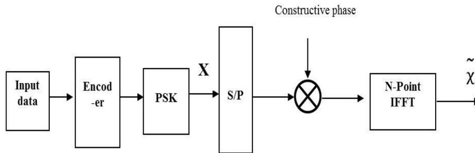
Fig. 2 Architecture of exhaustive search SLM
