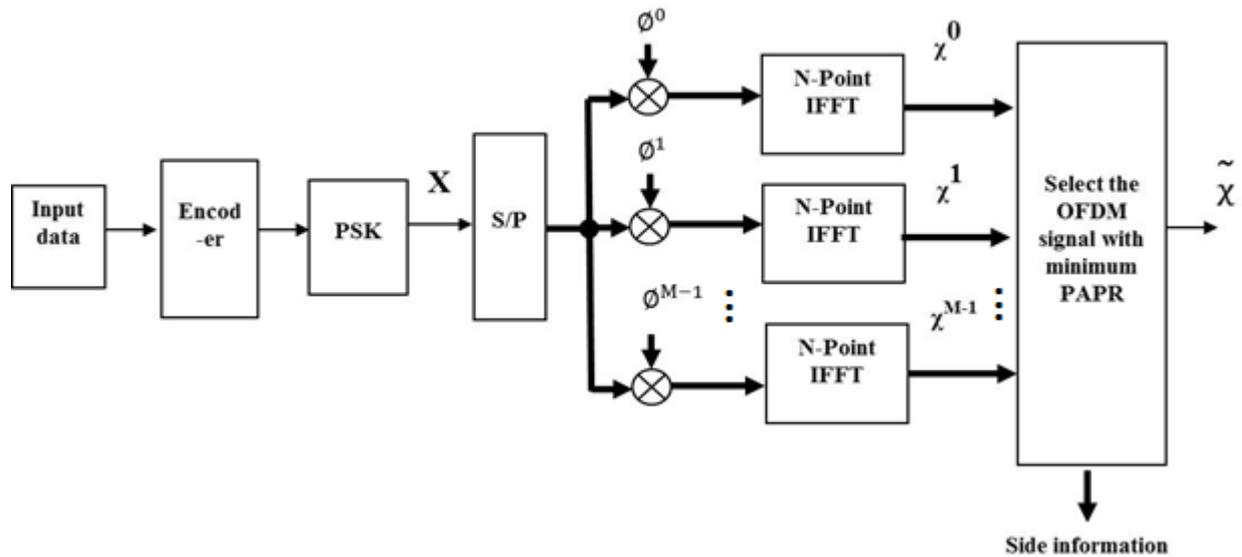
Fig. 1 Architecture of conventional SLM
