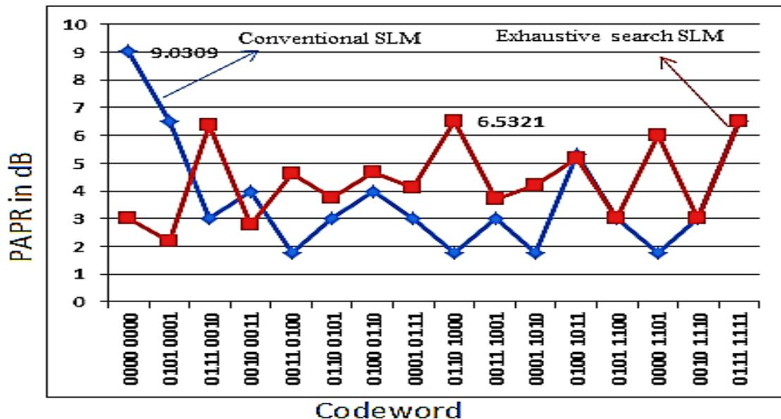
Fig. 4 PAPR values for conventional SLM and exhaustive search SLM with (8, 4) extended Hamming code
