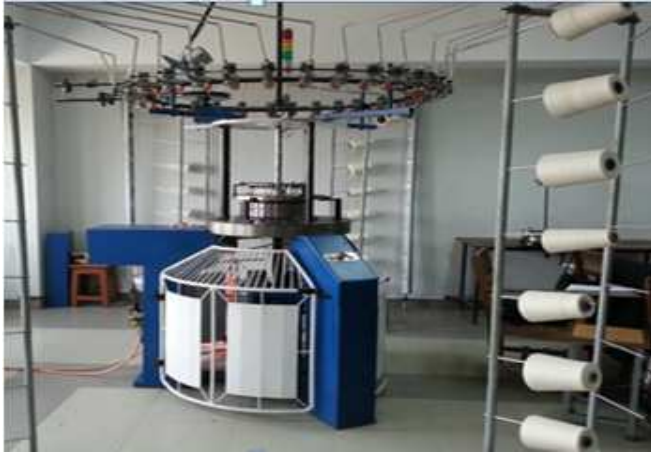
Fig. 1 Single jersey circular knitting machine
