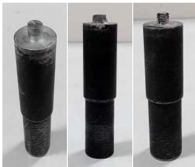
Fig. 2 Cylindrical, Square and Threaded Triangular pin profiles
