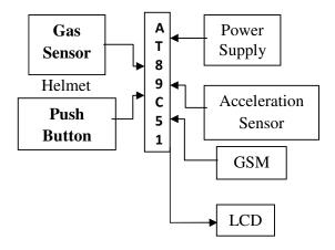
AT89C51 is an 8-bit microcontroller and belongs to Atmel's 8051 families. ATMEL89C51 has 4KB of Flash programmable and erasable read only memory (PEROM) and 128 bytes of RAM. It can be deleted and programmed to a maximum of 1000 times.
