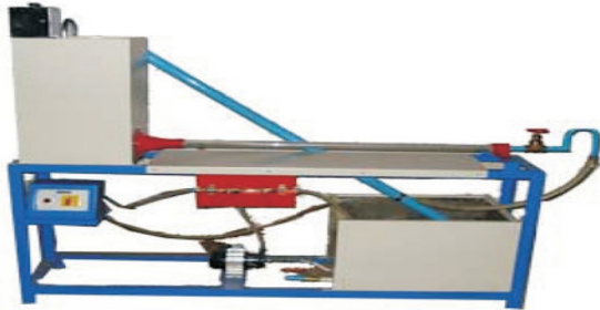
Fig:1 VERIFICATION OF REYNOLDS NUMBER BY DENSITY METHOD
