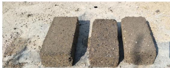
Fig. 2 Bricks after Demoulding
