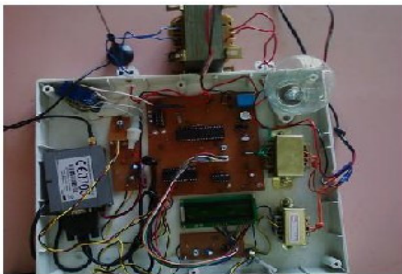
Fig.4. Hardware kit of transformer monitoring and protection.
