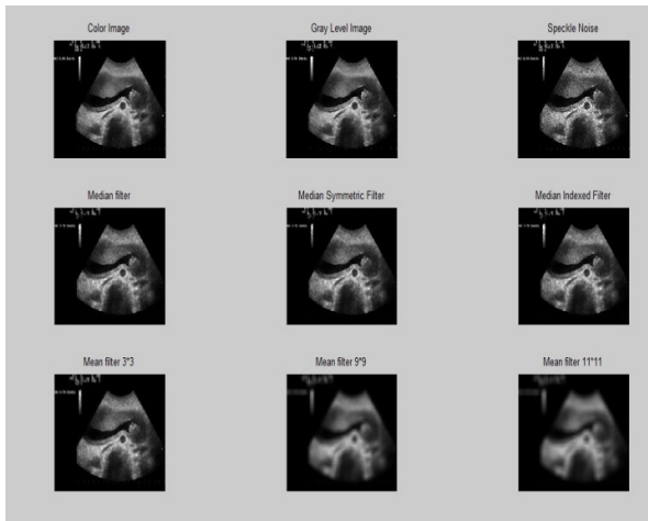
Fig.3 Ultrasound denoising using mean and median filter in matlab
