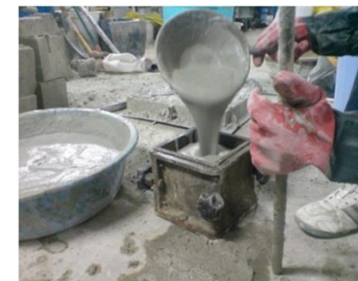
Figure 7: The produced foam concrete samples.
