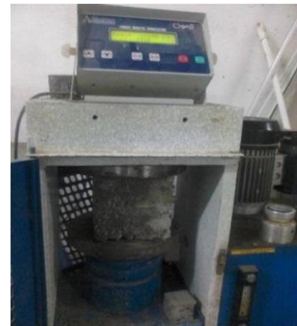
Figure 5: Compressive strength test of the first sample.
