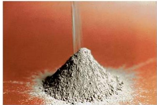
Figure 1: Micro silica used in concrete mix design.
