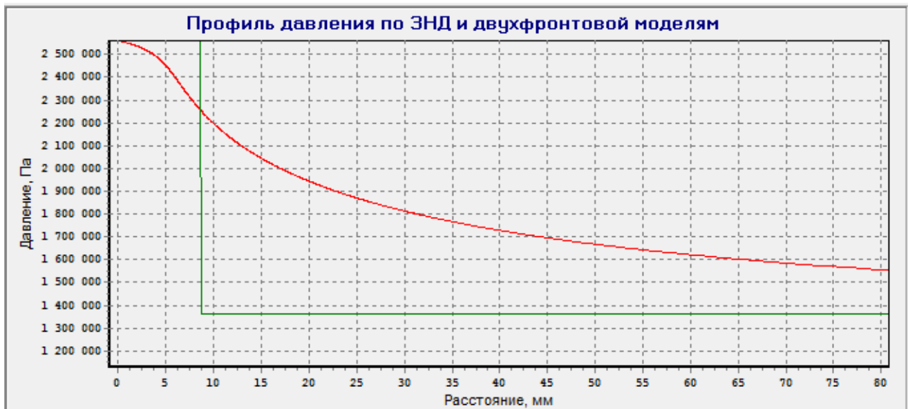
Fig. 3 – Pressure profile for stoichiometric hydrogen-oxygen mixture
