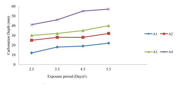
Fig. 4 Carbonation depth vs exposure period after air-curing [14].
