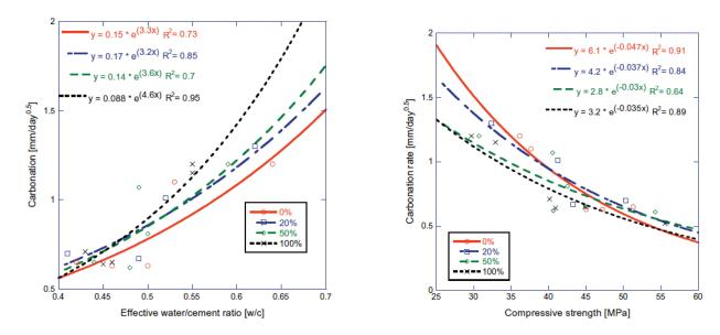
Fig. 13 Relationship between the rate of carbonation and compressive strength with different levels of RCA [50]
