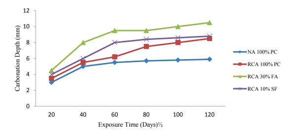
Fig. 14 Carbonation depth vs exposure time for different levels of RCA substitution with addition of fly ash and silica fume [47]
