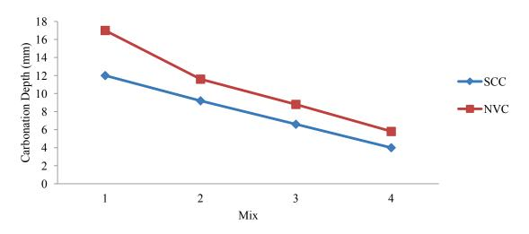
Fig. 19 Carbonation depth after 42.5 months of accelerated carbonation [24]
