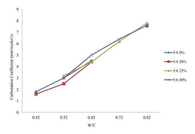
Fig. 1 Carbonation coefficient vs w/c ratio and fly ash content [4].
