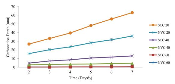
Fig. 20 Carbonated depth vs sq. root of time for SCC and NVC having different grades of strength for an exposure period of 7 days [58]
