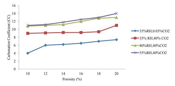
Fig. 11 Carbonation coefficient vs porosity for natural and CO<sub>2</sub> enriched environment with different levels of relative humidity (RH) [29].
