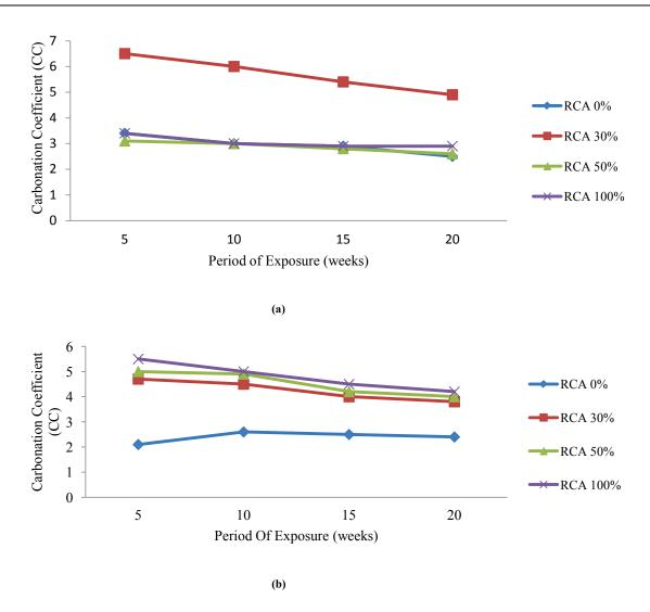
Fig. 17(a & b) Relationship showing carbonation coefficient-exposure period for concrete mix made with different levels of RCA with and without replacement of fly ash [49].
