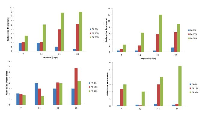
Fig. 16 Carbonation depth measured at different exposure period for 21 day curing with varying levels of levels of RCA; (a) 0% (b) 30% (c) 60% (d) 100% with low levels of fly ash [52].
