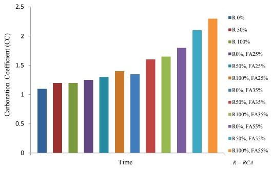
Fig. 15 Carbonation coefficient after 10 years of natural exposure for altered percentages of RCA with different levels of fly ash [51].
