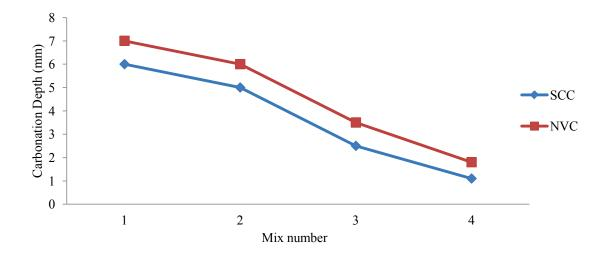
Fig. 18 Carbonation depth after 9 months of accelerated carbonation [24]
