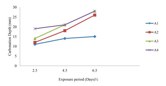
Fig. 5 Carbonation depths vs exposure periods after water-curing [14].
