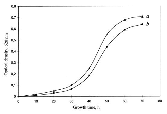
Figure 4: Growth dynamics of *H. halobium ET 1001* under various experimental conditions: *a*) – SM-medium; *b*) – peptone medium. Growing conditions: the incubation period: 4–5 days, temperature: +35 °C, the illumination under monochrome light at  $\lambda$  = 560 nm
