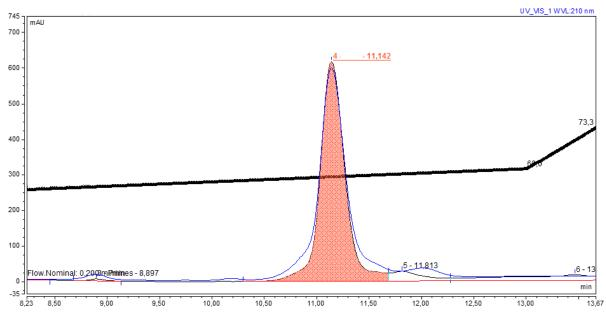
Figure 6: The GPC-chromatogram of the BR sample after purification (shaded as orange shows the separated protein): GPC (150×10 mm) column; stationary phase: Sephadex G-200 ("Pharmasia",
