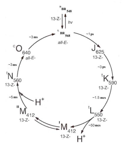
Figure 3: Photocycle scheme of BR (aqueous solution, pH = 7.2; t = +20±25 °C). Latin numbers J, K, L, M, N, O denote spectral intermediates of BR. <sup>1</sup>M and <sup>11</sup>M represent spectral intermediants of *meta*- bacteriorhodopsin with the protonated (<sup>1</sup>M) and deprotonated (<sup>11</sup>M) aldimine bond. L and D denote dark and light forms of pigments. The subscripts correspond to the position of the absorption maximum in the photocycle intermediates (nm)
