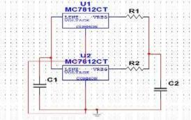
Please note that in this circuit diagram, I have used resistors for load balancing purpose so the output of this voltage regulator circuit may slightly inaccurate. Both resistors should be minimum 15 Watt or above.
