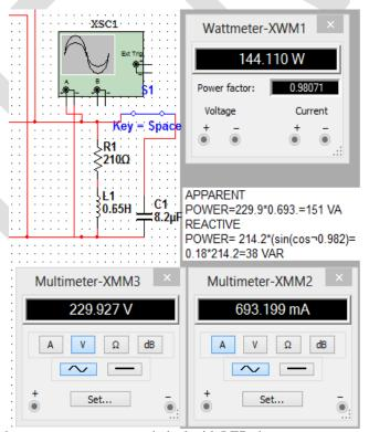
The above figure shows when compensator was switched with LED the apparent power reduces. **Conclusion:**
