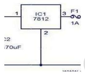
In electronics markets, 7812 is sold under various names such as 7812a, 7812act, 7812t and lm7812. All of them are almost identical with a little to no differences at all. 7812 input voltage range is 14V to 35V. Exceeding the voltage range may damage the IC. Given bellow is 7812 pin diagram to make the pin out connections clear in case you want to do some experiments.
