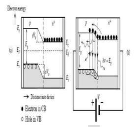
To understand the principle, let's consider an unbiased p-n junction (Figure 1 shows thep-n energy band diagram). The depletion region extends mainly into the p-side. There is a potential barrier from Ec on the n-side to the Ec on the p-side, called the built-in voltage, V0.
