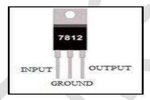
If you hold upside down (pins up) and the IC number is facing you then the left pin will be the voltage regulator output, the center pin will be ground and the right pin will be the voltage input pin. Under my experience, the maximum safe current you can get from one 7812 IC is 1A.
