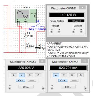
This above figure shows when the model was simulated and the results were shown, as shown the apparent power required for model was 214.2 VA
