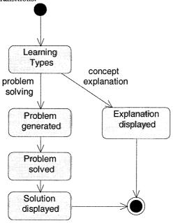
Figure 5. The State-Chart Diagram for the Learning Use-Case
