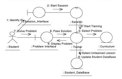
Figure 8. A Collaboration Diagram for the Training Use-Case
