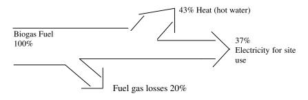
Figure 4. Sankey diagram showing energy flow at STW
