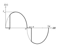
Figure 5. Nonlinear-load current
