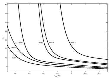
Figure 6. Operating time values versus rms values of current for all modes
