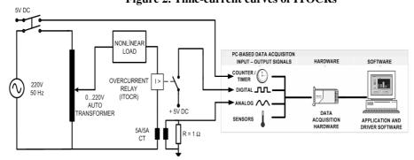
Figure 3. Test system configuration
