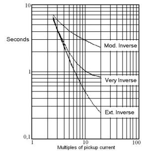
Figure 2. Time-current curves of ITOCRs
