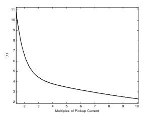
Figure 4. Time-current characteristic of ITOCR for sinusoidal current
