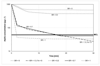
**Figure 1.** Effect of KMnO<sub>4</sub> on oxidation of As(III) in the presence and absence of  $Fe^{2+}$ . Initial  $Fe^{2+}$  concentration: 10 mg L<sup>-1</sup>.
