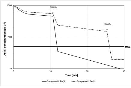
**Figure 2.** Effect of initial oxidation state of Fe and time of  $KMnO_4$  addition on As(III) oxidation. In the case of Fe<sup>3+</sup>,  $KMnO_4$  addition after 15 minutes and in the case of Fe<sup>2+</sup>,  $KMnO_4$  addition after 15 minutes and 30 minutes. (MCL: Maximum Concentration Level).
