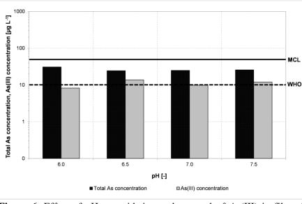
**Figure 6.** Effect of pH on oxidation and removal of As(III) in filtered samples  $(0.45 \ \mu\text{m})$  at SR=1 using KMnO<sub>4</sub>+Al<sub>2</sub>(SO<sub>4</sub>)<sub>3</sub> solution.
