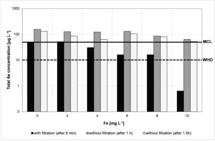
**Figure 5.** Removal of As in filtered and non-filtered samples with different Fe concentrations after treatment to pink color of the  $KMnO_4+Al_2(SO_4)_3$  solution.
