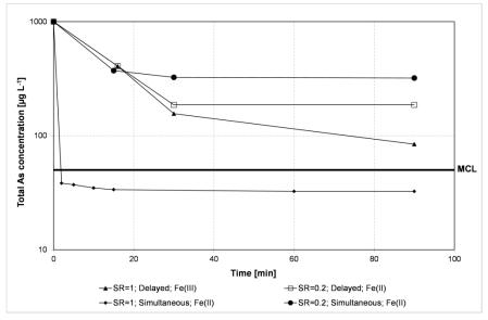
**Figure 3.** Effects of initial oxidation state of Fe and time of  $KMnO_4$  addition on total As removal in filtered samples (0.45 µm).
