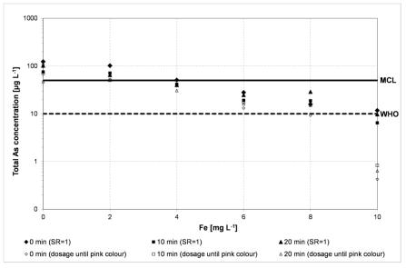
**Figure 4.** Influence of initial Fe concentration, time of sedimentation and amount of KMnO<sub>4</sub>+Al on As removals at an initial As(III) concentration of 500  $\mu$ g L<sup>-1</sup> in filtered samples (0.45  $\mu$ m). Filled symbols represent the addition of KMnO<sub>4</sub> and Al equal to SR = 1 and open symbols represent a slight excess of KMnO<sub>4</sub> and Al until a pink color appears. 0, 10 and 20 min represent sedimentation times.
