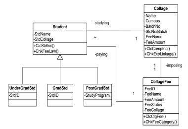
Figure 9: Object Class Diagram of the Fees Subsystem.
