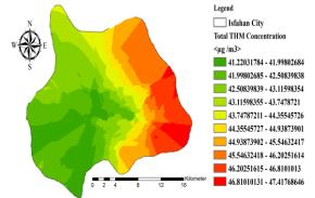
Fig. 3: Zoning of THMs contamination by kriging in IWDN
