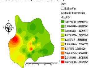
Fig. 4: Zoning of residual chlorine concentration by IDW in IWDN
