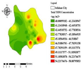
Fig. 2: Zoning of THMs contamination by IDW in IWDN
