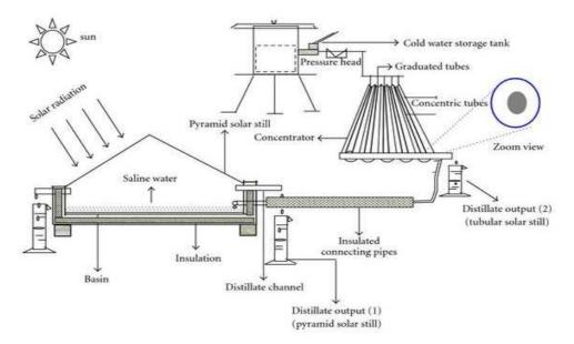
Figure 5: Cross Sectional View of Coupled Tubular and Pyramid Solar Still.
