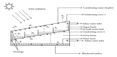
Figure 3: The Cross-Sectional View of Solar Still Has Double Basin Glass
