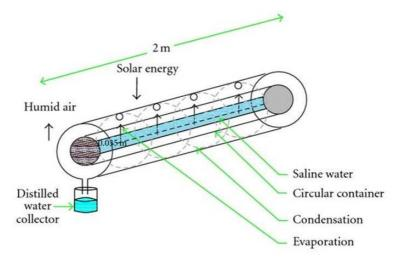
Figure 2: A Solar Still in Tubular Form
