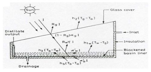
Figure 1: Diagram of a Conventional Single Slope Solar Still
