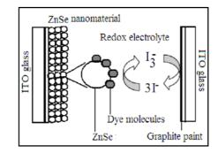
Figure 1: Schematic Overview of a Dye Sensitized Solar Cell
