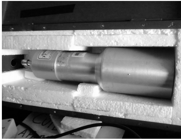
Figure 1: Nal (Tl) Scintillator/ PMT in Aluminum Housing and Amplifier
