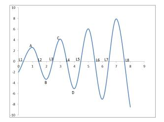
The roots of equation (4) above are a complex conjugate with positive real part. From stability, we saw that when the real part of a complex root is positive, this makes the system unstable. The trajectory of such a solution explodes as time increases.
