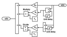
Figure 7: Discrete form PID Controller structure
