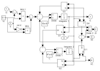
Figure 3: Simulink Model of buck converter (Power stage)
