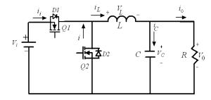
Figure1: Power stage of synchronous buck converter
