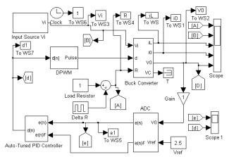
Figure 12: Closed loop Simulink model of buck converter with Fine-tuned Discrete PID Controller
