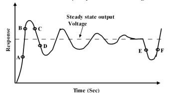
Figure 9: Typical closed loop response of DC-DC converter as second order (Under damped) system
