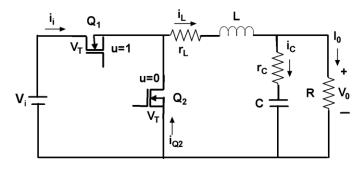
Figure 2: Buck converter with non-ideal components
