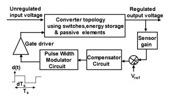
Figure 5: Detailed block diagram of closed loop control of switching converter topologies
