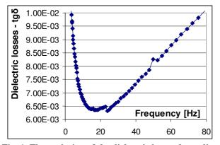
Fig. 1. The evolution of the dielectric losses depending on frequency on the suspension of *Saccharomyces cerevisiae* with 5% sucrose.
