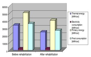
Fig. 7. Comparative energy performance for electricity and heating, final and primary energy consumption before and after rehabilitation
